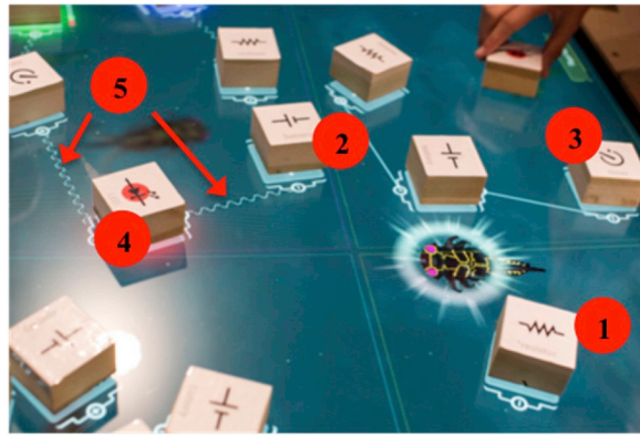
Fig. 2. Participants assemble virtual circuits using wooden blocks that represent resistors (1), batteries (2), timers (3), and different colored LEDs (4). Participants make circuit connections (5, depicted as lines on the tabletop) by bringing the positive and negative terminals of the blocks (augmentations displayed on the table) in contact with one another. Creating a successful circuit (i.e., one that has the correct ratio of resistors, batteries, and LEDs) causes the LEDs to glow and lure the fish attracted to that light out for cataloging.
