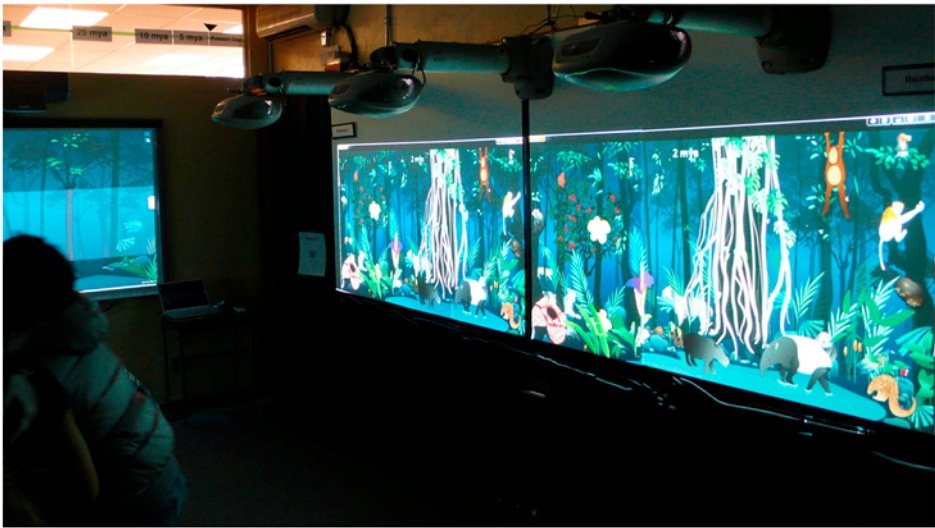
Figure 2. Three projectors make up a sidewall of EvoRoom.
