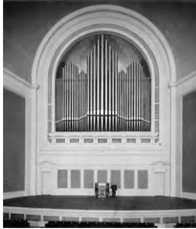
FIGURE 1.2 Festival Hall of the Panama-Pacific International Exposition in San Francisco, California, was home to opus 500 of the Austin Organ Co. built in 1915. This four-manual symphonic instrument of 110 stops had five manual divisions (Great, Swell, Choir, Solo, Echo) and Pedal with pipes voiced on five, ten, fifteen, or twenty-five inches of wind pressure (127 mm, 254 mm, 381 mm, 635 mm). Symphonic organs were hidden behind simple pipe fronts or screens, as here in a vaguely Jugendstil or Art Nouveau style, or in more elaborate cases to match ecclesiastical interiors, or even behind decorative fronts or architectural grills with no pipes at all. After the 1915 fair, the organ was moved to the new Civic Auditorium in San Francisco. A handful of changes were made to the instrument over the years, but it was infrequently heard in later decades before it was damaged in the 1989 Loma Prieta earthquake. The organ has been repaired and is presently in storage. Courtesy Vic Ferrer Productions, Inc.
