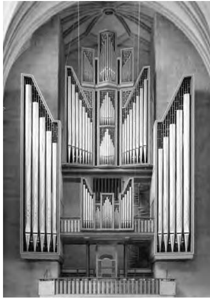
FIGURE 1.5 Rudolf von Beckerath (1907–76) was one of the leading organbuilders of the German Orgelbewegung and his firm completed the large four-manual instrument with mechanical key and electric stop actions in the church of St. Andreas, Hildesheim, Germany in 1966. From bottom to top, the manual divisions are readily distinguished (with the pitch of the lowest Principal rank): 8' Rückpositiv, 4' Brustwerk (behind Swell shades), 16' Hauptwerk, and 8' Oberwerk. The 32' Pedal is on the gallery rail, a situation also found on historic instruments of North Germany. With its geometric case, the Hildesheim organ is clearly a product of its time, although the wing-shaped side towers add an attractive and fresh element to an otherwise functional design. The organ survives in its original condition. Courtesy Fa. Beckerath Orgelbau and St.-Andreas Gemeinde, Hildesheim.
